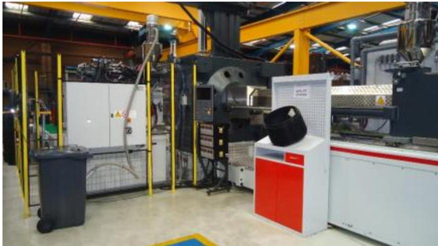
The moulding cycle involves injection of the main riser body, then transfer to a second cavity using a full servo 3-axis robot. After formation of the TPE seal, the same robot removes the finished component, whilst replacing it with the next riser body.
